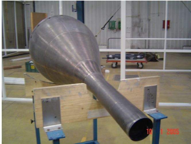
Fig. 3. Low frequency liner in engine centerbody.
